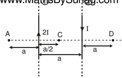
**Sol.** (i) Let us call  $\vec{B}$  due to (1) and (2) as  $\vec{B}_1$  and  $\vec{B}_2$  respectively. Then at A :  $\vec{B}_1$  is  $\odot$  and  $\vec{B}_2$  is  $\otimes$
