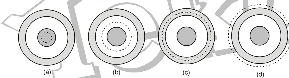
A cross-section of the cable is shown in figure. Draw a circle of radius  $x$  with the centre at the axis of the cable. The parts a, b, c and d of the figure correspond to the four parts of the problem. By symmetry, the magnetic field at each point of a circle will have the same magnitude and will be tangential to it. The circulation of  $B$  along this circle is, therefore,
