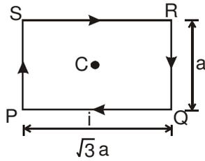
**Sol.** It is clear that 'B' at 'C' due all the wires is directed  $\otimes$ . Also B at 'C' due PQ and SR is same. Also due to QR and PS is same
