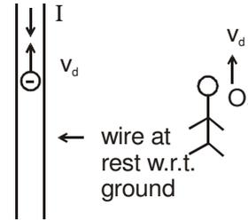
So, w.r.t.  $O_1$  electrons will produce zero magnetic field but +ve ions will produce +ve same  $\vec{B}$  due to the current carrying wire does not depend on the reference frame (this true for any velocity of the observer).
