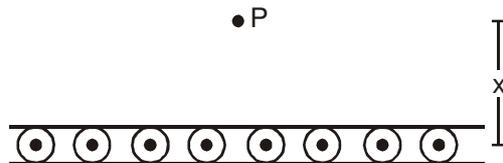
**Sol.** Consider two strips  $A$  and  $C$  of the sheet situated symmetrically on the two sides of  $P$  (figure). The magnetic field at  $P$  due to the strip  $A$  is  $B_a$  perpendicular to  $AP$  and that due to the strip  $C$  is  $B_c$  perpendicular to  $CP$ . The resultant of these two is parallel to the width  $AC$  of the sheet. The field due to the whole sheet will also be in this direction. Suppose this field has magnitude  $B$ .
