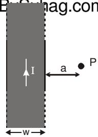
**Sol.** To find 'B' at 'P' the sheet can be considered as collection of large number of infinitely long wires. Take a long wire distance 'x' from 'P' and of width 'dx'. Due to this the magnetic field at 'P' is 'dB'
