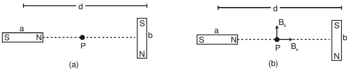
**Sol.** The point P is in end-on position for the dipole a and in broadside-on position for the dipole b. The magnetic field at P due to a is  $B_a = \frac{\mu_0}{4\pi} \frac{2M}{(d/2)^3}$  along the axis of a, and that due to b is  $B_b = \frac{\mu_0}{4\pi} \frac{M}{(d/2)^3}$  parallel to the axis of b as shown in figure. The resultant field at P is, therefore.
