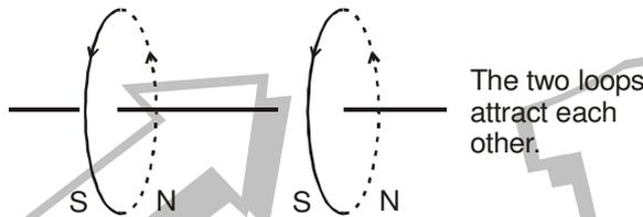
$$B_{\text{axis}} = \frac{\mu_0 N I R^2}{2(R^2 + x^2)^{3/2}} \approx \frac{\mu_0 N I R^2}{2x^3} \text{ for } x \gg R = 2 \left( \frac{\mu_0}{4\pi} \right) \left( \frac{I N \pi R^2}{x^3} \right)$$
