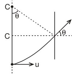
**Ex. 27** What should be the speed of charged particle so that it can't collide with the upper wall? Also find the coordinate of the point where the particle strikes the lower plate in the limiting case of velocity.
