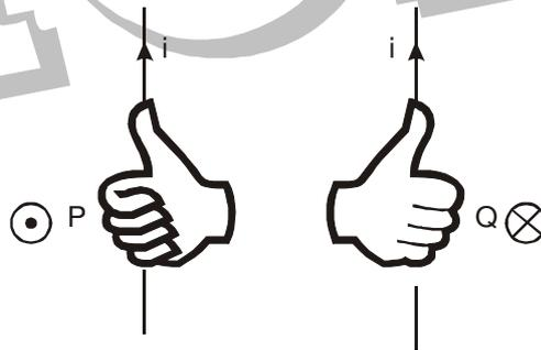
We can draw magnetic field lines on the pattern of electric field lines. A tangent to a magnetic field line gives the direction of the magnetic field existing at that point. For a straight wire, the field lines are concentric circles with their centres on the wire and in the plane perpendicular to the wire. There will be infinite number of such lines in the planes parallel to the above mentioned plane.
