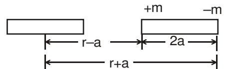
$$\therefore F_{res} = F_1 - F_2 = 2\left(\frac{\mu_0}{4\pi}\right) m_1 m \left[ \left(\frac{1}{(r-a)^3}\right) - \left(\frac{1}{(r+a)^3}\right) \right] = 2\left(\frac{\mu_0}{4\pi}\right) \frac{m_1 m}{r^3} \left[ \left(1 - \frac{a}{r}\right)^{-3} - \left(1 + \frac{a}{r}\right)^{-3} \right]$$
