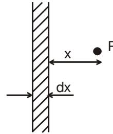
**Ex. 14** In the figure shown a large metal distributed current I is kept in the yz plane with its centre at the origin. Find magnetic field at a point P (d, 0, 0)
