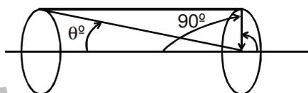
**Q. 6** A thin solenoid of length 0.4 m and having 500 turns of wire carries a current 1A; then find the magnetic field on the axis inside the solenoid.
