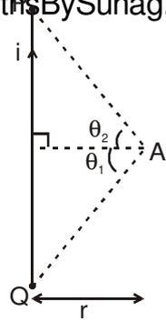
**Direction :** Due to every element of 'PQ'  $\vec{B}$  at A is directed in wards. So its resultant is also directed in wards. It is represented by (x)
