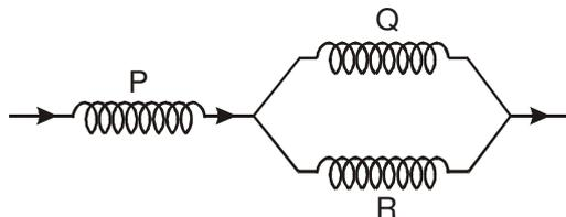
**Sol.** As the solenoids are identical, the currents in  $Q$  and  $R$  will be the same and will be half the current in  $P$ . The magnetic field within a solenoid is given by  $B = \mu_0 ni$ . Hence the field in  $Q$  will be equal to the field in  $R$  and will be half the field in  $P$  i.e., will be  $1.0$  T.
