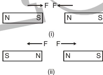
The poles of the same magnet do not come to meet each other due to attraction. They are maintained we cannot get two isolated poles by cutting the magnet from the middle. The other end becomes pole of opposite nature. So, 'N' and 'S' always exist together.
