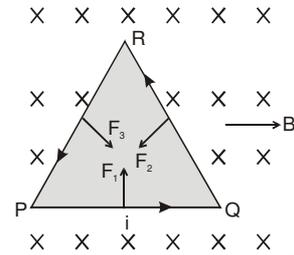
The forces  $\vec{F}_2$  and  $\vec{F}_3$  on QR and RP can also be obtained similarly. Both the forces are 1.0 N directed perpendicularly to the respective sides and towards the inside of the triangle.
